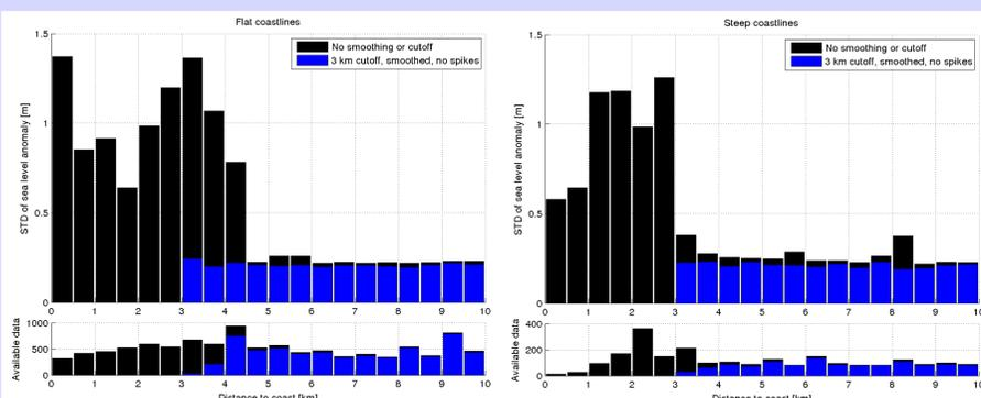
Figure 4. Standard deviation of sea level anomaly as measured by the satellite as a function of distance to the coast for flat coastlines (left) and steep coastline (right), using the ALES retracker. The black bars represent data with no coastal cutoff, spike removal, or smoothing. The blue bars represent a 3 km cutoff distance, smoothing with a 3 km window, and spike removal.
