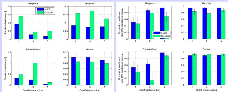
Figure 5. Standard deviation of the difference between in situ observations and the nearest available satellite data (left, note varying scale) and corresponding correlation coefficient with 95% confidence intervals (right) for the 4 tide gauges marked in figure 1. For each station, statistics are shown for the ALES and CoastAlt retrackers, using 1, 3, and 5 km cutoff distance to the coast for the satellite data. All satellite data have been smoothed with a 3 km window and spikes removed.
