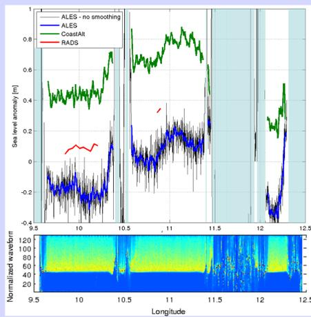
Figure 2. Top: example of sea level anomaly, Envisat cycle 27 for selected study area. Thick lines: cutoff distance 3 km from coast, 3 km smoothing, and spikes removed. Thin lines: no cutoff, smoothing, or spike removal. Shaded areas are on land. Bottom: corresponding normalized waveform.
